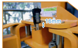
16mm thickened steel plate
