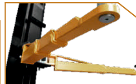
Second and third supporting arms with 20% higher strength than standard lifts, suitable for sports cars with ultra-low chassis designs
